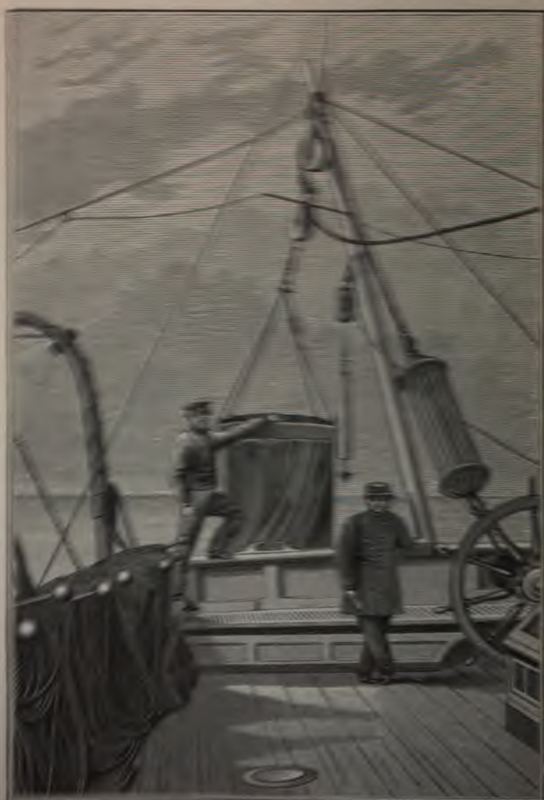
FIG. 45.—The main derrick of the 'Porpoise,' showing the 'accumulator,' the derrick, and the mode of hauling the net.
